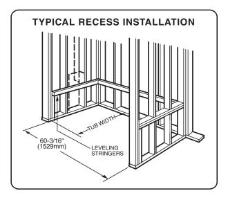
**B.)** Check level front to back and side to side, shim as necessary. To secure the tub to wood studs, use drywall screws with flatwashers or roofing nails immediately above the flange of the bath. To secure the tub to steel studs, use 4" drywall screws and flatwashers.
